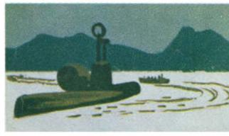
Under the dangerous arctic ice, the Nautilus can move along with assurance. The A-sub is guided by sonar which determines the location of outside objects by gauging sound echoes
